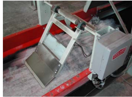
A sensor like the sled pictured here can provide an advance signal to turn drying temperature up or down in response to moisture..
