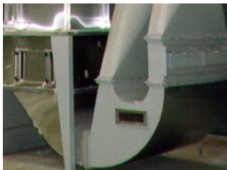
Left: A seed cotton skimmer to double drying air volume.
