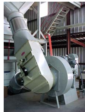
The Electric Banjo can be used on unloading fans or on drying system pull fans to increase operating air volume 30%
