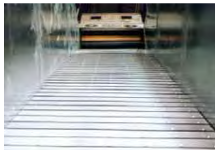
A Lint Slide Grid for economical lint moisture restoration
