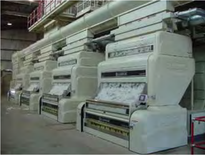
A typical Conditioning Hopper System
