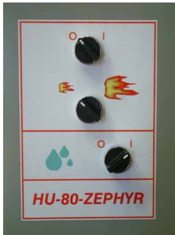
The Zephyr's Selector Switch Controls
