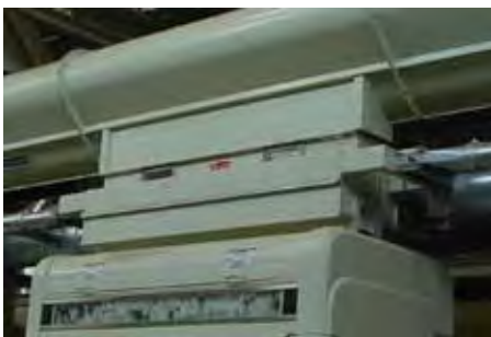
A Conditioning Hopper for seed cotton moisture restoration
