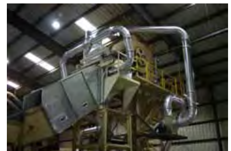
A Steamroller for powerful and efficient lint moisture restoration
