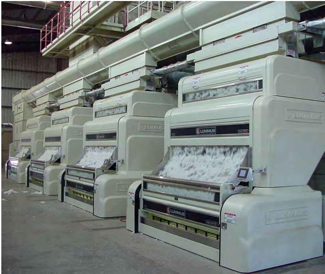
Conditioning Hoppers in operation at a gin running at over 60 bales per hour.
